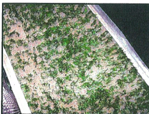
Highest Flow and Final Channel Condition after Testing (no significant loss of mortar mix)
